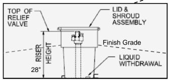
fig. A. Detail of dome
