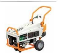
Generator manufacturer Generac has introduced two portable propane generators in recent years. The LP3250 produces 3,250 watts and operates for 9 hours on a 20-pound propane tank, while the LP5500 produces 5,500 watts and offers a 4.75-hour run time with a 20-pound tank. Both models incorporate a tank holder into the frame itself, so the propane tank sits securely out of the way.
