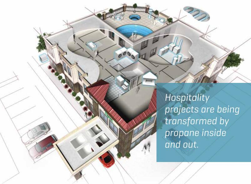
Combined heat and power (CHP). CHP systems create electricity while providing supplemental heat for a hotel's swimming pool and radiant heating system. Because of their year-round hot water loads for laundry, pool heating, guest rooms, radiant heating, and more, hospitality buildings are an ideal candidate to utilize this rapidly growing technology, which can also provide electricity during power outages.
