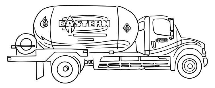
A bobtail is a special vehicle built to hold and deliver propane.
